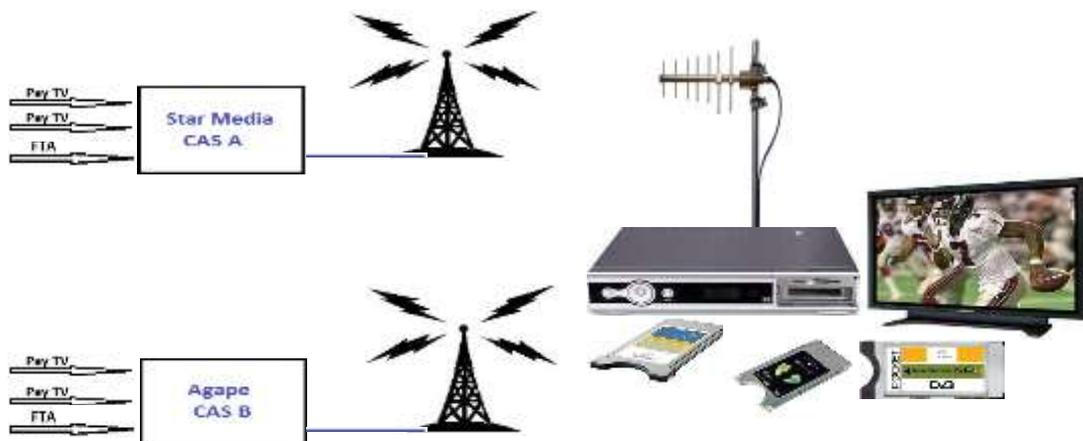
**Figure 5:** Indicates different CAS received with the same STBs or iDTV but allowing flexibility of changing detachable CAM from different service providers.
